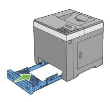
NOTICE: Do not use excessive force on the tray. Doing so could damage the tray or the inside of the printer.
